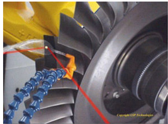
The Air Force ManTech Program, working with General Electric Aircraft Engines and LSP Technologies, Inc., developed an emerging technology, called laser shock peening, as a potential solution to increase the durability of titanium fan blades and decrease the sensitivity to foreign object damage. Laser shock peening uses a high-energy laser pulse to impart an intense shock wave into the surface of metal parts. The shock wave creates deep compressive residual stresses which greatly improve fatigue properties and toughness.
